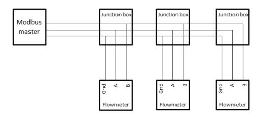
Shielded twisted pair should be used. Connection of a third wire between the master and slave should be done to limit the common mode voltage that can be impressed on the slaves inputs. The required cable quality depends on the total cable distance, the number of nodes and the environmental influences. A local contractor can help you select the right cable for your application.
